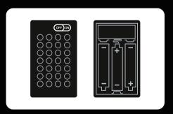
4.Check that the power switch on the battery box is on and that the "+" and "-" poles of the battery are correctly placed (using new batteries) and ensure that the upper and lower connections to the "+" and "-" poles of the power switch are installed correctly.
