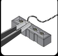
2.Use tweezers to hold the connector on both sides.
