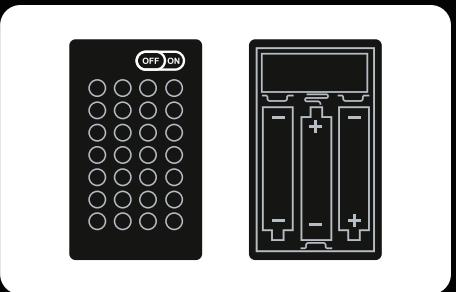
4. Check that the power switch on the battery box is on and that the "+" and "-" poles of the battery are correctly placed (using new batteries) and ensure that the upper and lower connections to the "+" and "-" poles of the power switch are installed correctly.
