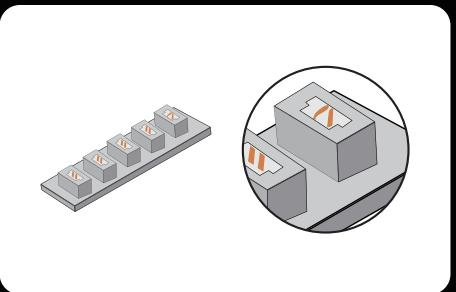
3. Check the internal pins of the connector sockets. The internal pins of a properly working connector port should be straight. If the small pins are bent, they may be considered faulty ports.
