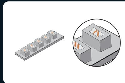
3. Check the internal pins of the connector sockets. The internal pins of a properly working connector port should be straight. If the small pins are bent, they may be considered faulty ports.
