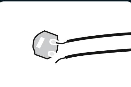
2. Check if the wires are disconnected or broken from the solder joints.
