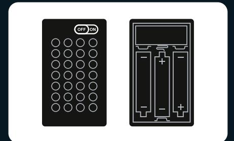
4. Check that the power switch on the battery box is on and that the "+" and "-" poles of the battery are correctly placed (using new batteries) and ensure that the upper and lower connections to the "+" and "-" poles of the power switch are installed correctly.
