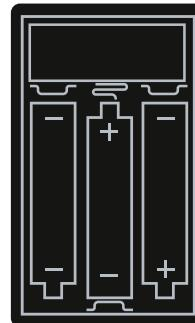
4. Check that the power switch on the battery box is on and that the "+" and "-" poles of the battery are correctly placed (using new batteries) and ensure that the upper and lower connections to the "+" and "-" poles of the power switch are installed correctly.
