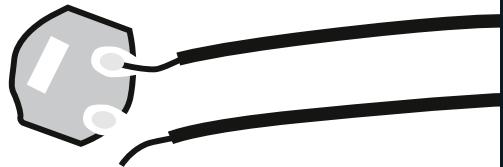
2. Check if the wires are disconnected or broken from the solder joints.
