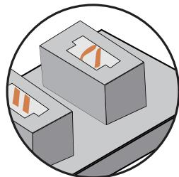
3. Check the internal pins of the connector sockets. The internal pins of a properly working connector port should be straight. If the small pins are bent, they may be considered faulty ports.
