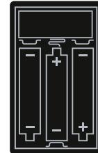
4. Check that the power switch on the battery box is on and that the "+" and "-" poles of the battery are correctly placed (using new batteries) and ensure that the upper and lower connections to the "+" and "-" poles of the power switch are installed correctly.
