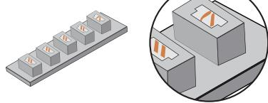
3. Check the internal pins of the connector sockets. The internal pins of a properly working connector port should be straight. If the small pins are bent, they may be considered faulty ports.
